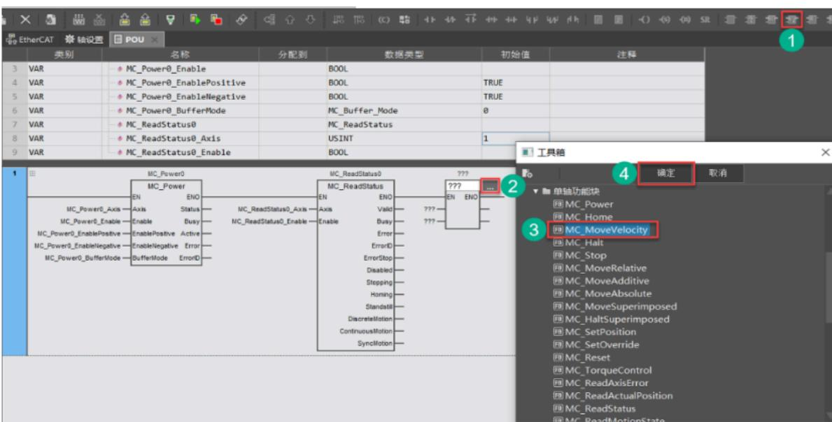
④Add network and insert MC\_Halt function block
