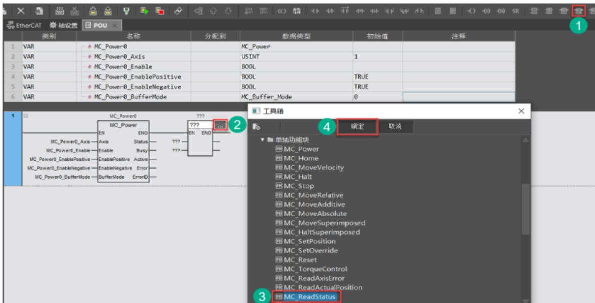
③Insert the MC\_MoveVelocity function block
